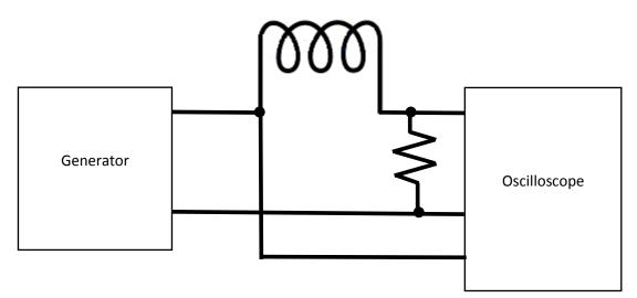
Although the wire was pretty long, the distance from the generator to the load resistor was not longer than 0.1 meter.
